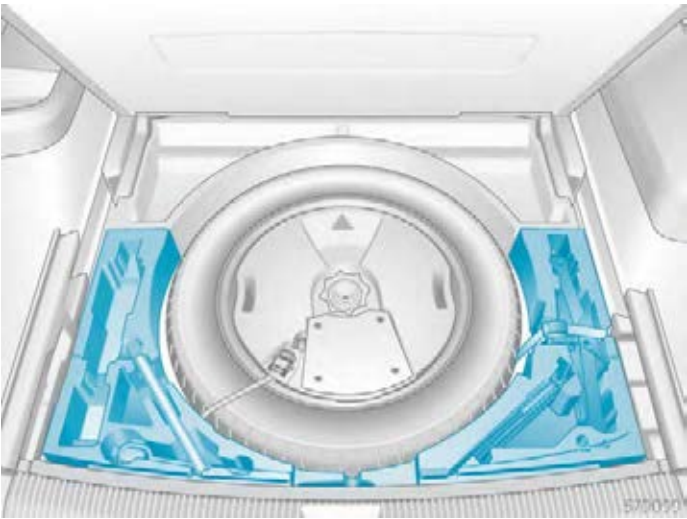
Figure 1. Spare tire and vehicle tools under the trunk floor
