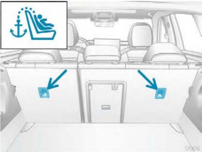
Figure 1. ISOFIX child seat with top fastening cord.
