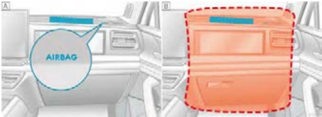
Figure 2. Installation location and inflation range of the front passenger airbag.
