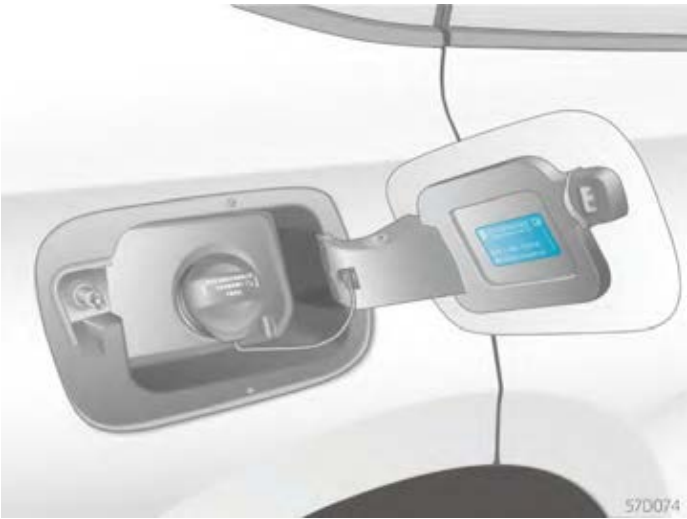
Figure 1. Label inside the fuel filler cap.
