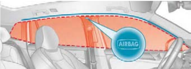
Figure 1. On the left side of the car: the installation position and inflation range of the head airbag.
