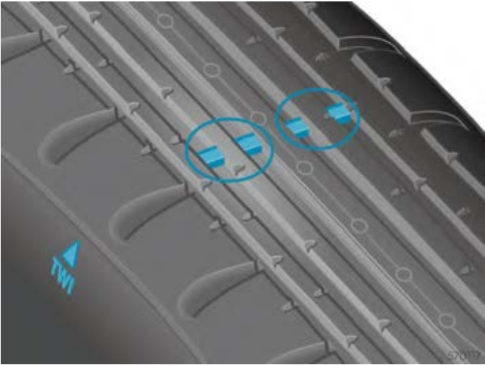
Figure 1 Tire tread wear indicators
