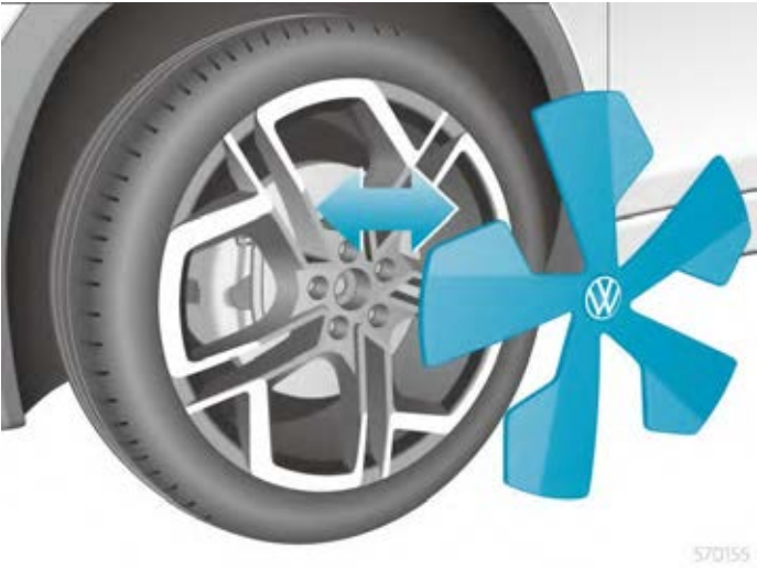
Figure 1. Removing and reinstalling the wheel cover.
