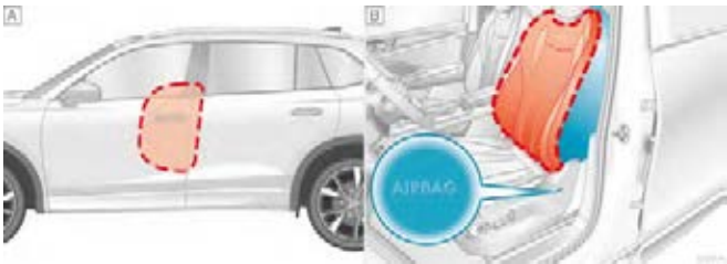
Figure 1 A. Left side of the vehicle - inflation range of the side airbag; B. Left front seat side - installation position and inflation range of the side airbag.
