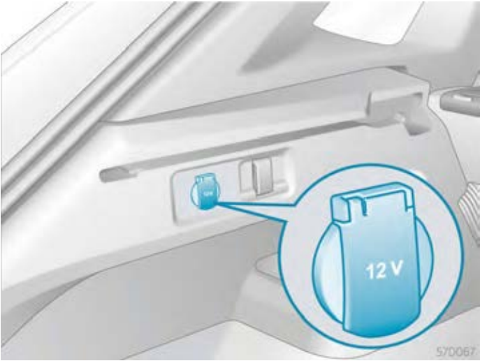
Figure 1 12V power socket
