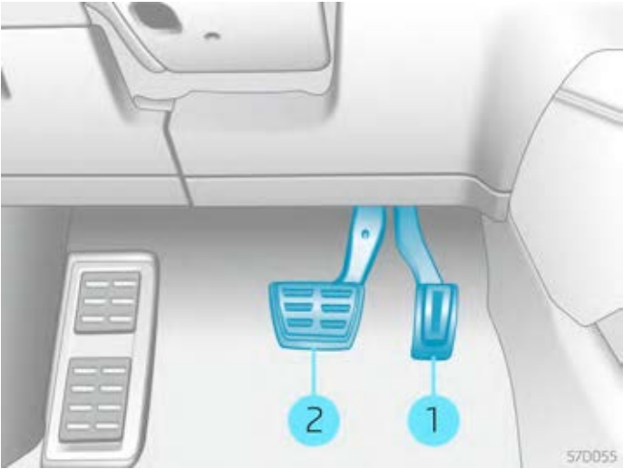
Figure 1. Pedals on a car with an automatic transmission: ① Accelerator pedal ② Brake pedal
