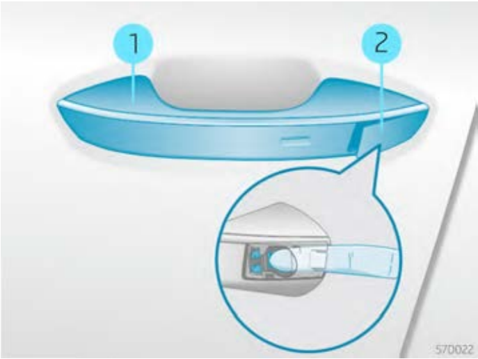
Figure 1. Removing the cover from the inside of the driver's door lock.
