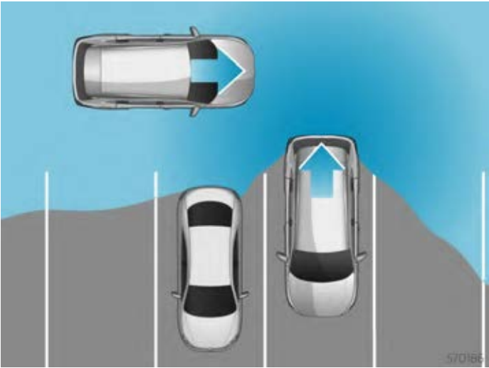
Figure 1. Surveillance range around the vehicle when it leaves the parking space (illustrative diagram)
