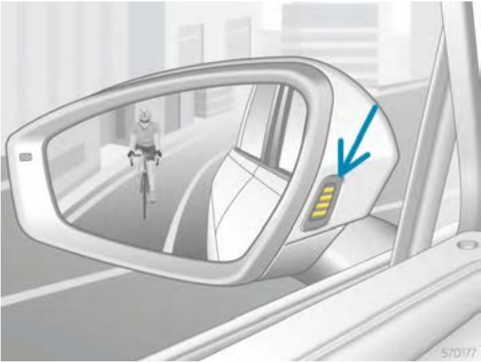
Figure 1. Exit warning system display in the exterior rearview mirror housing (illustration)
