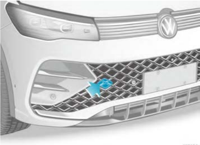
Figure 1. Right front of the bumper: Removing the cover plate.
