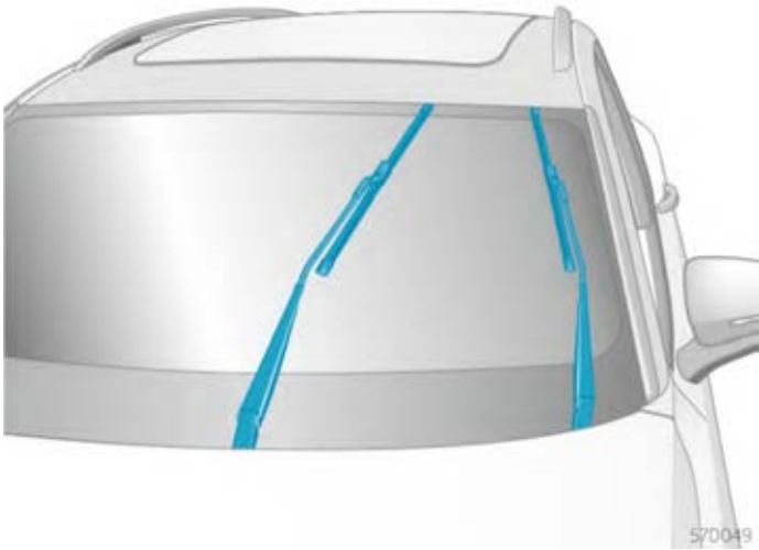
Figure 1. Wiper blade in maintenance position.
