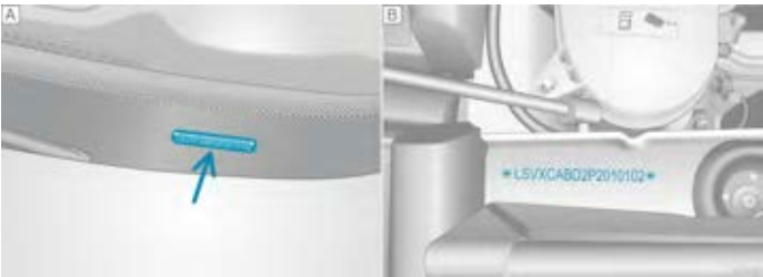
Figure 1 A. Vehicle Identification Number (VIN) B. Location of the VIN stamp in the engine compartment
