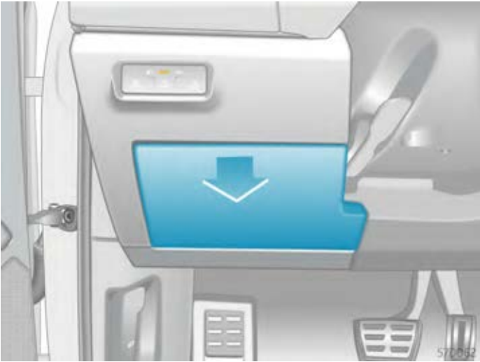
Figure 1. Fuse box cover on the driver's side dashboard.
