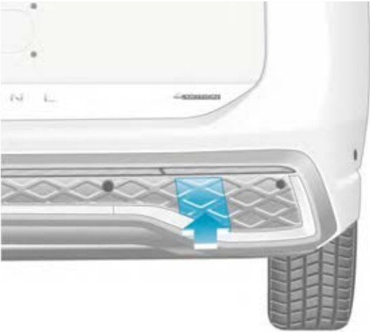
Figure 1. Right rear of the bumper: Removing the cover plate.
