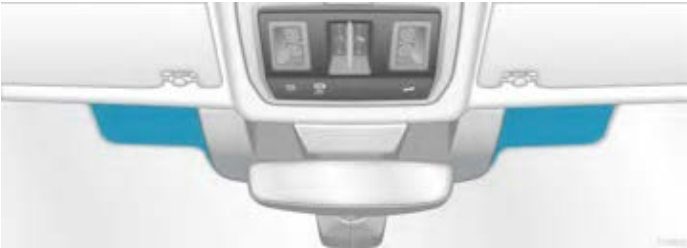
Figure 1. Infrared reflective metal-coated windshield with communication window (blue area).
