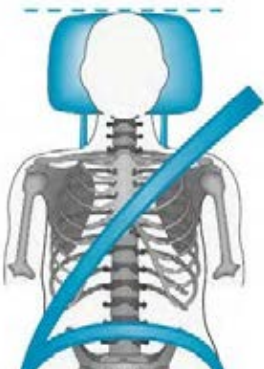
Figure 1. Maintain a distance of at least 25 cm between the driver and the steering wheel.
