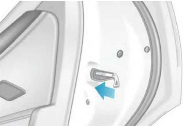
Figure 1. Emergency locking device inside the right rear door lock.
