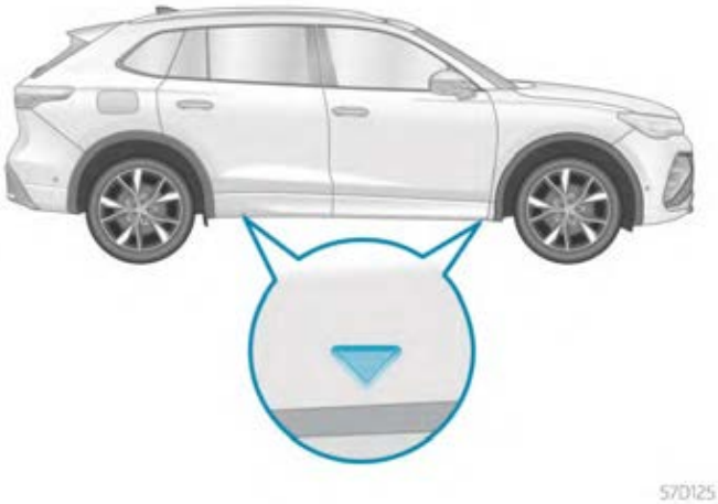
Figure 2. Support points of a car jack
